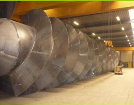
With a diameter of 4.30 meters and a length of 22 meters, these are probably the biggest jack-screws in the world for such an application. The screws were placed in a pump installation and a hydro-electric power plant on the Albert Canal at the lock complex of Ham.
