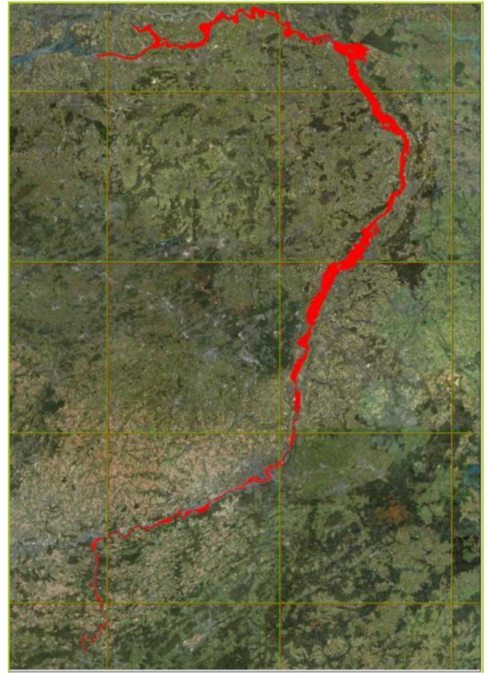
Flood extension for Q100 in the time horizon 2071-2100. Map from Givet (France) to Keizersveer (the Netherlands)
